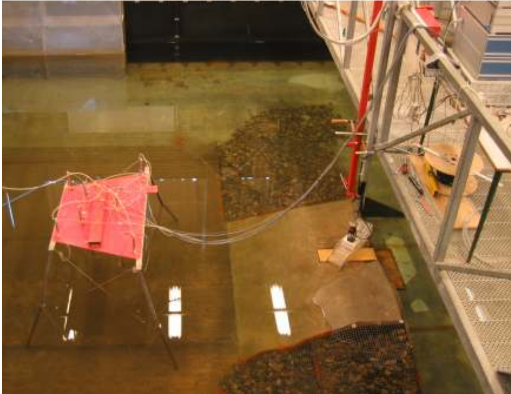
Figure 3. Tests setup. The 1:60 model is placed on an artificial cliff and turned of 45° in order to simulate the 45° wave's attack angle.
