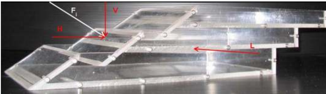
Figure 2. Decomposition of forces on the SSG model.
