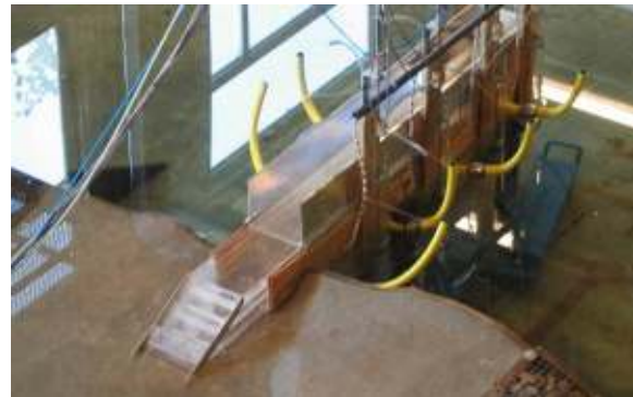
Figure 9: Model for 3D overtopping tests.
