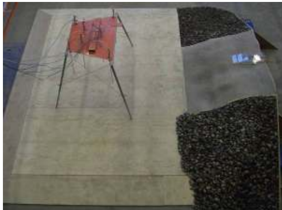
Figure 3: Plexiglas model on the reproduction of the cliff at Kvitsøy; in front the seven resistive probes.
