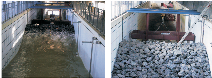
Figure 4. Installation of the overtopping tank in GWK. The tank was placed behind the structure and consisted of an inner and outer tank.
