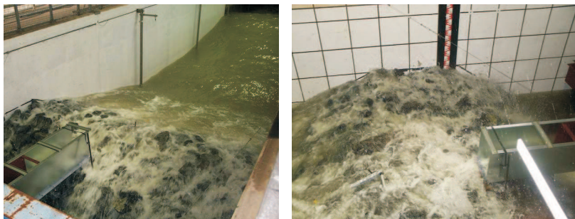
Figure 8. The momentum of the water is too little to cross the width of the crest. The water sinks almost immediately between the stones.
