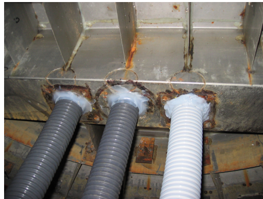
(c) View of the model from underneath: exhausting pipes and air chambers
