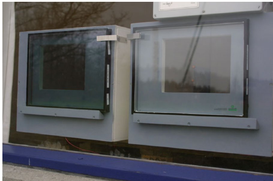
Figure 1. Photograph showing the scale models and their window opening covered by glazing sample.
