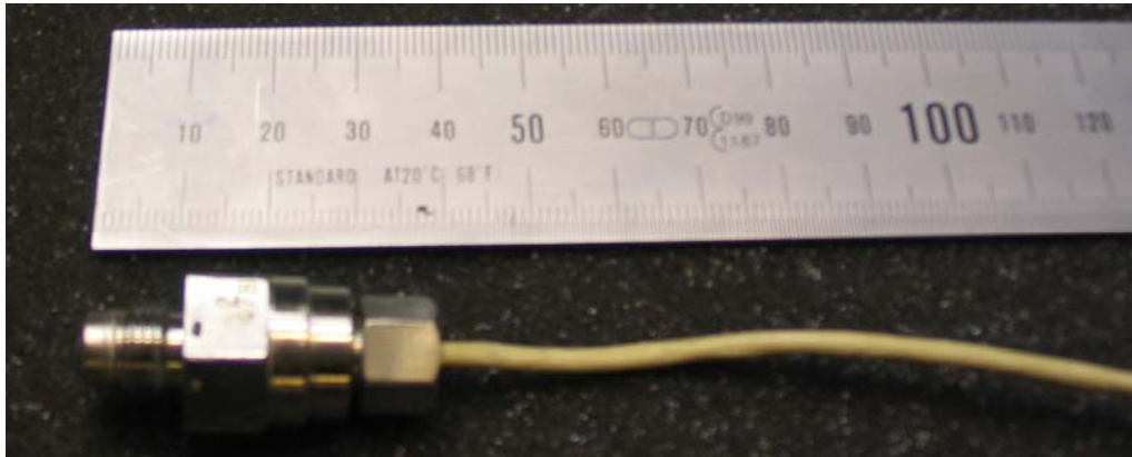
Figure 13. Kulite Semiconductor pressure cell.
