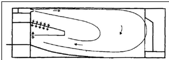
FIG. 5. Horizontal ventilation principle as used in theatres and cinemas.
