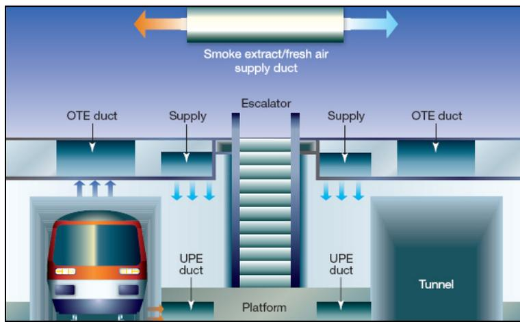
FIG. 6. Layout of modern subway ventilation system. Source: Arup (London).
