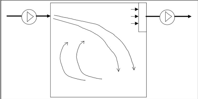
FIG. 2. Ventilation system using the mixed principle.
