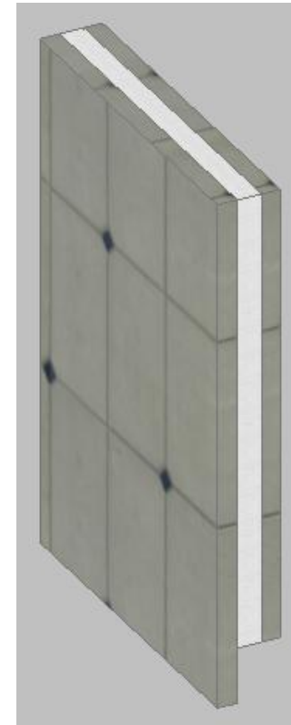
Figure 7: Wall Offset of concrete part and insulation
