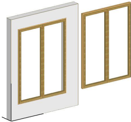
Figure 14: Window in Wall – Window replaces wall
