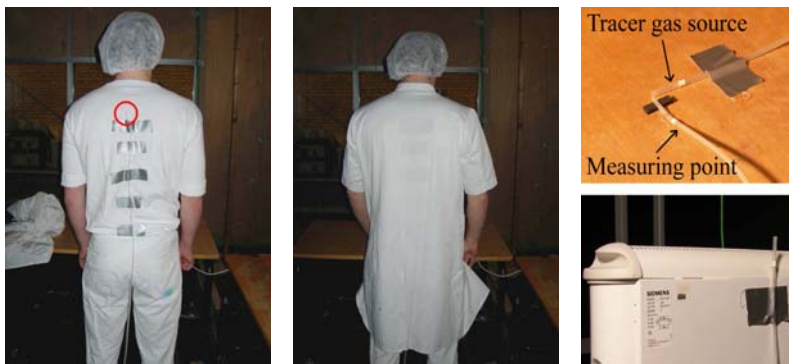
Figure 4. Three different tracer gas contaminant sources. Left and centre: Source at the back of a person (with and without coat). Upper right: Source on Table 1 (the tracer gas source and the measuring point are not applied at the same time). Lower right: Source above Convector 1.
