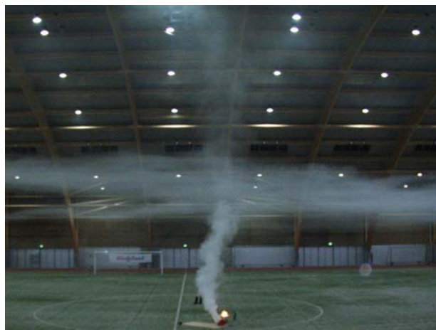
Figure 1. Smoke movement in a stadium hall. A vertical temperature gradient results in a stratified flow at a certain height.
