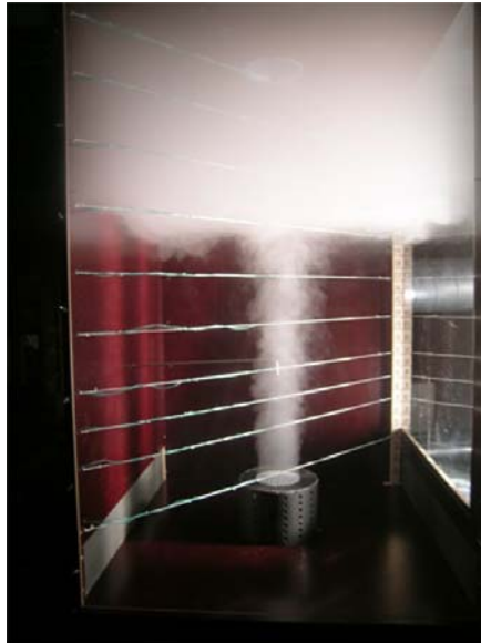
Figure 3. Stratification in the model with a high rate of heat release and an active smoke ventilation.
