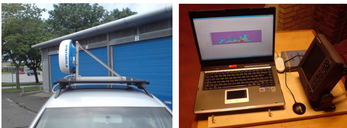
Figure 2. Left: The modified Furuno 1715 Microstrip Antenna mounted on top of a car. Right: data acquisition, communication and positioning system
