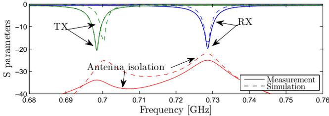
Fig. 5 Measured and simulated frequency responses in band 12.
