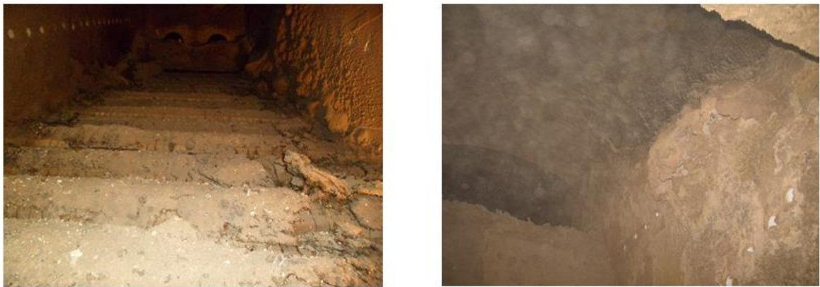
Figure 11: Melted slag on refractory walls.
