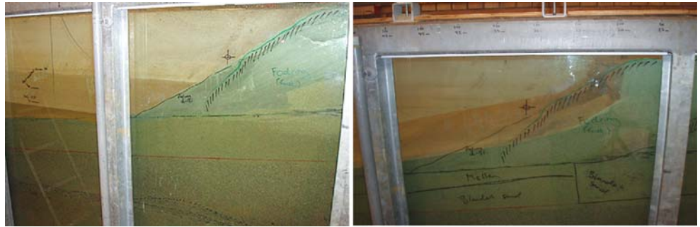
Fig. 11 Profile of the beach before (left) and after (right) the test (Holmgren et al. 2006a, b)
