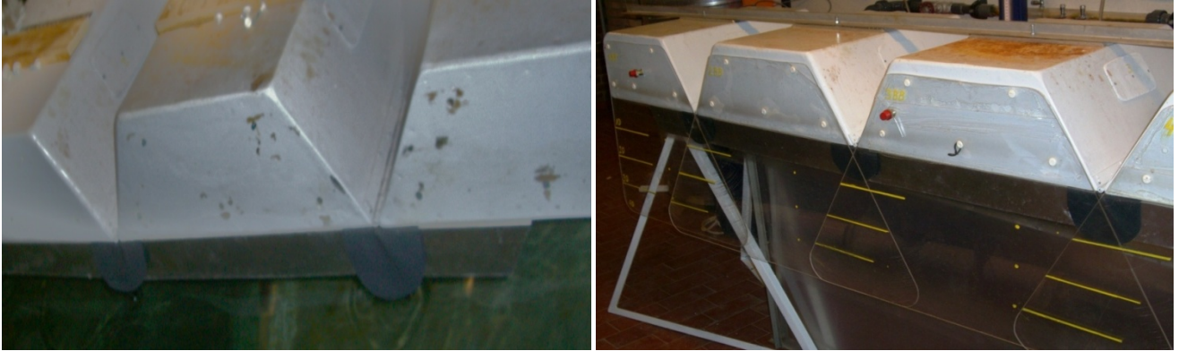
Figure 8: Left: The mini skirt referred to in the text is the metal skirt attached to the bottom of the WEC. It extends down approximately 8cm. Right: Original skirts extending down 40cm from the device.
