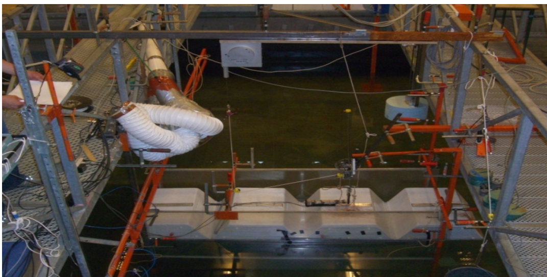
Figure 3: Set up of the Crest Wing WEC with fixed point PTO.
