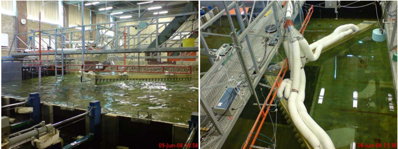
Figure 2 The LEANCON WEC 1:40 scale model in the deep 3-D wave basin at Department of Civil Engineering, Aalborg University.
