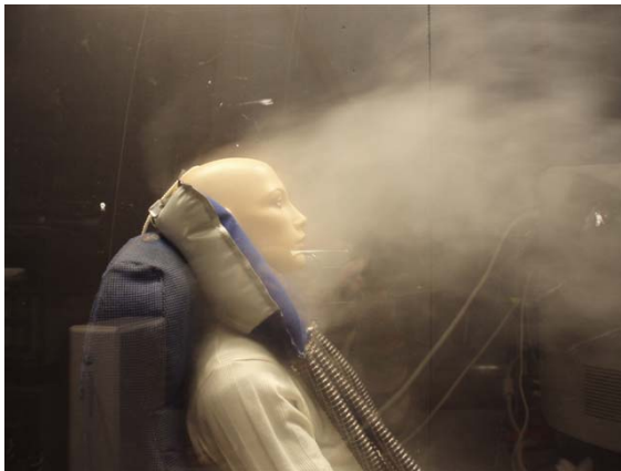
Figure 6. Smoke picture showing the distribution of “clean air” around the breathing zone of the manikin, and the effectiveness of the system. The draught is flowing from behind (180°).
