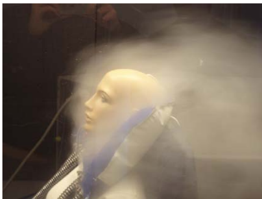
Figure 4. Smoke picture showing the distribution of “clean air” around the breathing zone of the manikin, and the effectiveness of the system. The draught is directed towards the face (0°).
