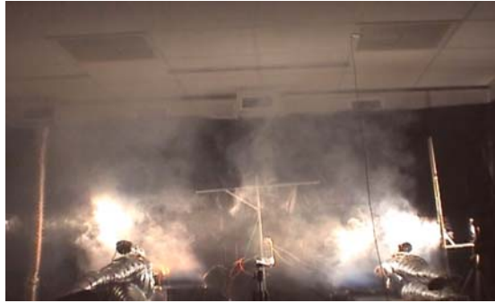
Figure 8. Smoke experiment with PV systems at both source and target manikins. The breathing zones are surrounded by smoke (clean air) and not disturbed by the supply flow from the general ventilation system in the room. T_{1,1} = 23\text{ }^{\circ}\text{C} , q_{PV} = 26\text{ l/s} .
