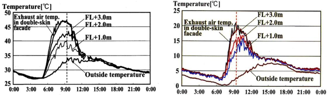
Figure 2.32. Air temperatures inside the DSF cavity for summer and winter
