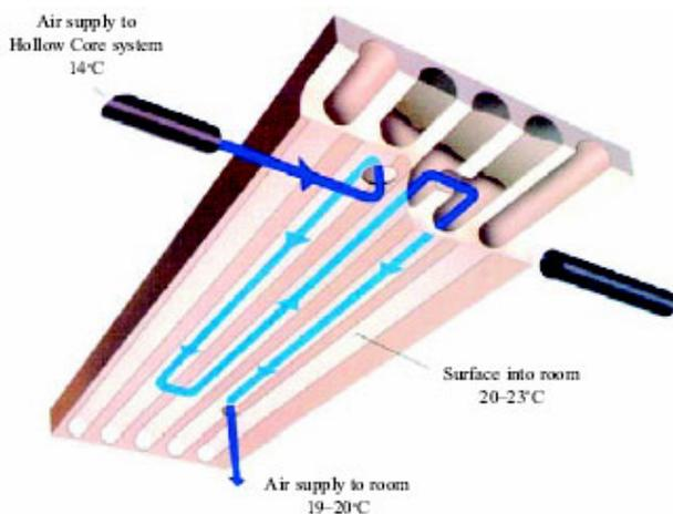
Figure 3.23 Principle of the TermoDeck® system.
