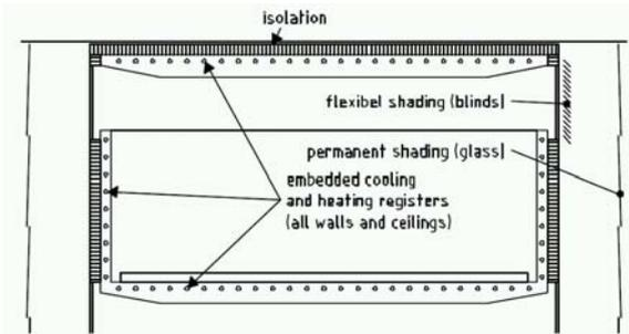
Figure 3.5 – Cross section of the building with activated concrete slabs and walls (Meierhans and Olesen 2002)
