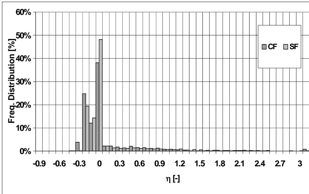
Figure 2.29. Frequency distribution of the pre-heating efficiency
