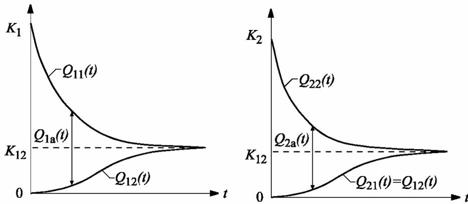
Figure 3.40 Character of the basic step-response heat fluxes.
