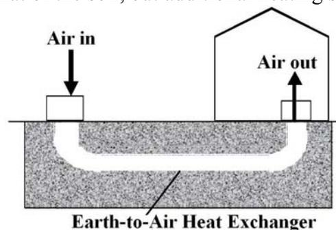
Figure 4.1. Building with an Earth-to-Air Heat Exchanger
