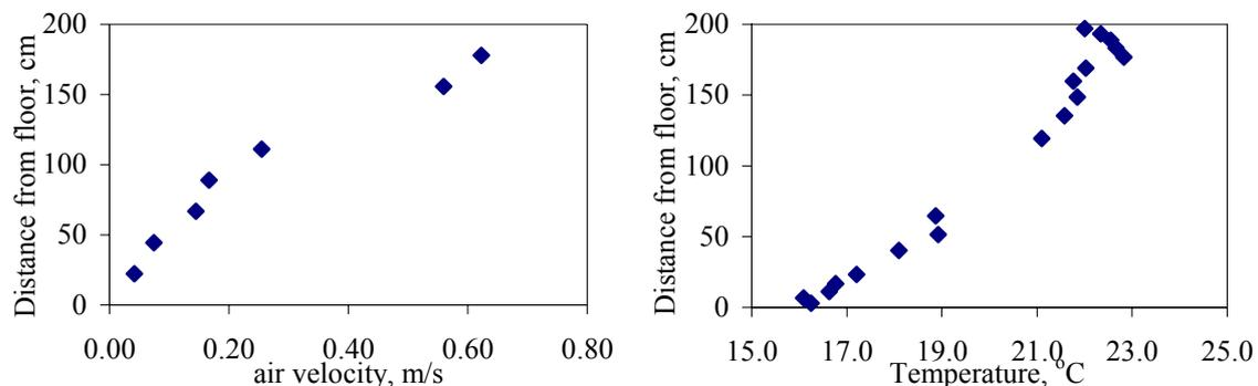
Figure 4.19. Measured vertical air velocity and temperature profiles in the air intake duct when the supply fan was off, the inlet air temperature was 23.7 °C, and the air flow rate was 0.931 m<sup>3</sup>/s. The location was 6.1 m from the supply fan on the middle plane. The duct end (refer to 5 in Figure 4.7) was partially sealed with the upper 1/3 area open.
