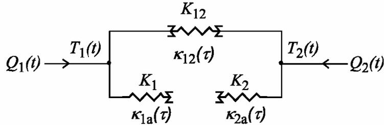
**Figure 3.3.1** Dynamic thermal network to represent the relations (1)-(2).
