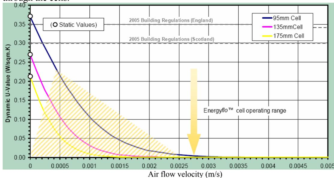
Fig 5.3 Variation of dynamic  $U$  value of walls incorporating Energyflo™ cells
