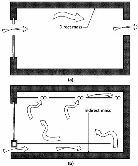
Figure 3.21 – Direct and indirect interaction thermal mass (CIBSE, 2001)
