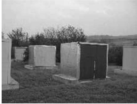
fig. 6.16: prototypes of box for experimental test of façades with PCM layer.
