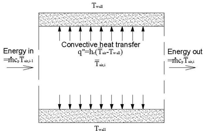
Figure 4.21. Heat convection between ETAHE walls and air
