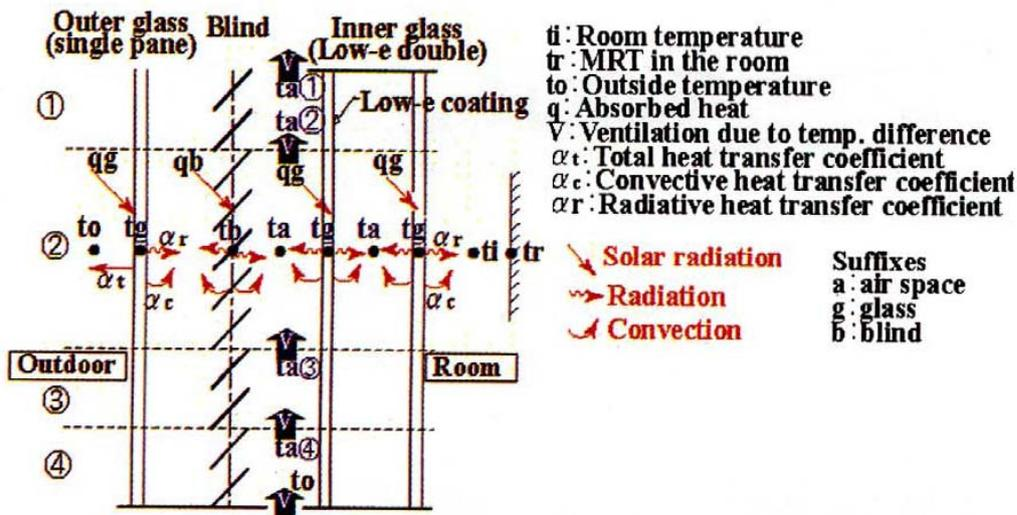
Figure 2.35 – “Window model” for a DSF façade [Takemasa, et al (2004)]
