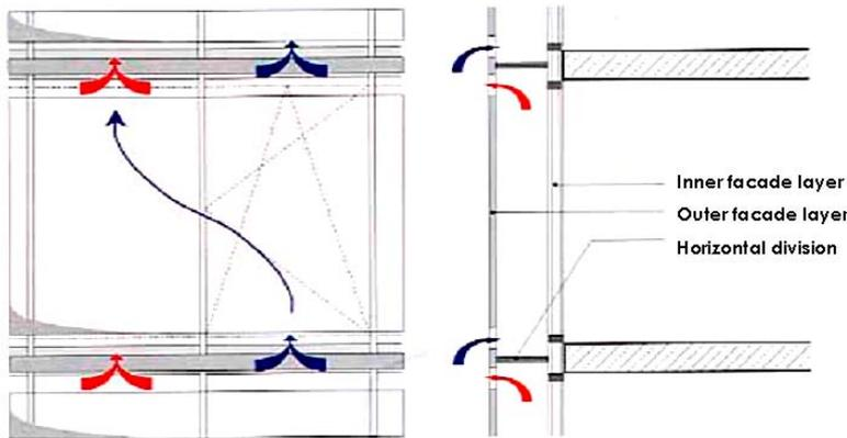
Figure 2.7. DSF – corridor configuration
