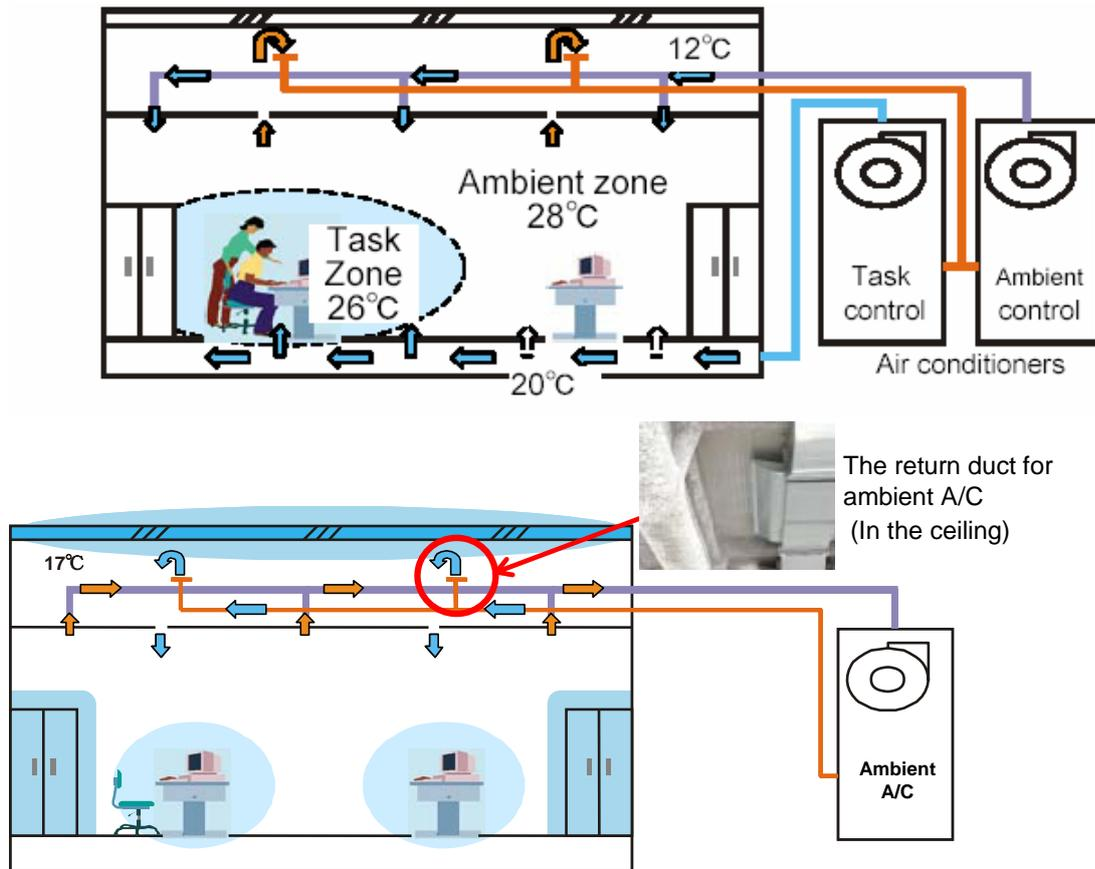
Figure 3.30 – Air conditioning system utilizing building thermal storage – operation principle
