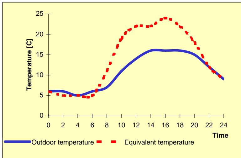
Figure 3.49 Comparison of outdoor or equivalent temperature during one day
