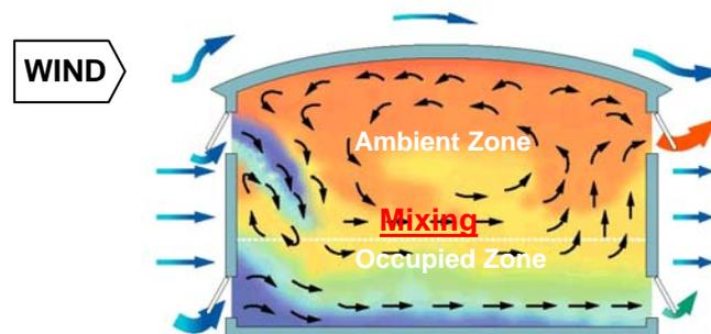
Figure 2.16. Natural ventilation using commonly used openings
