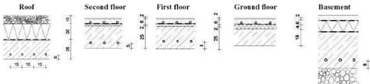
Figure 3.7 – Different positions of pipes as used in the ZUB in building Kassel, Germany (De Carli et al 2003)
