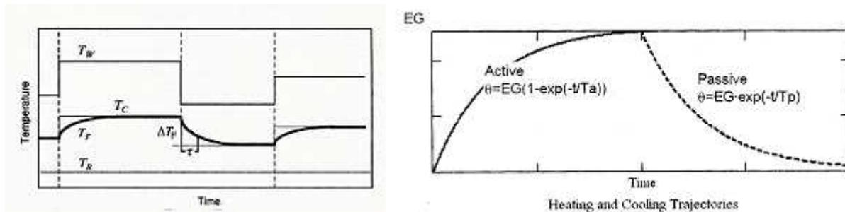
Figure 3.13 – left: The effect of stepwise varying water temperature  $T_W$  on the floor temperature  $T_F$ : asymptotically approaches the stationary floor temperature  $T_C$ . The symbol  $\tau$  is the response time of the floor mass (Rekstad et al. 2003); right: The typical heating and cooling trajectories (Chapman et al. 2004)
