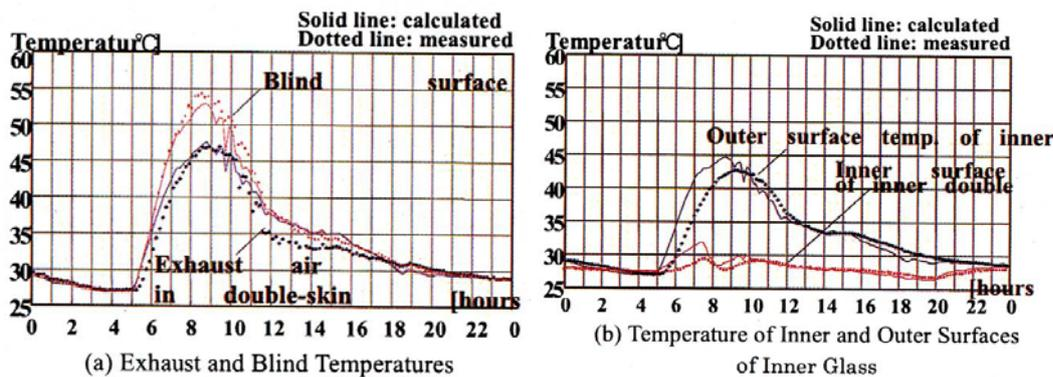
Figure 2.36. Comparisons between measured and calculated values
