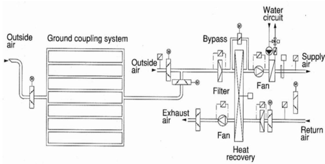
Figure 4.5. Ventilation system's components of Schwerzenbacherhof building (Hollmuller 2002).
