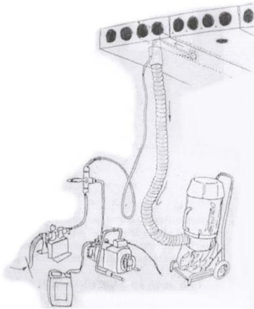
Figure 3.28 The Jet vent system for cleaning
