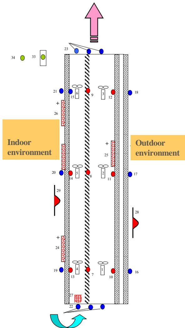
Figure 2.26. The monitored “climate façade” and the scheme of the experimental apparatus
