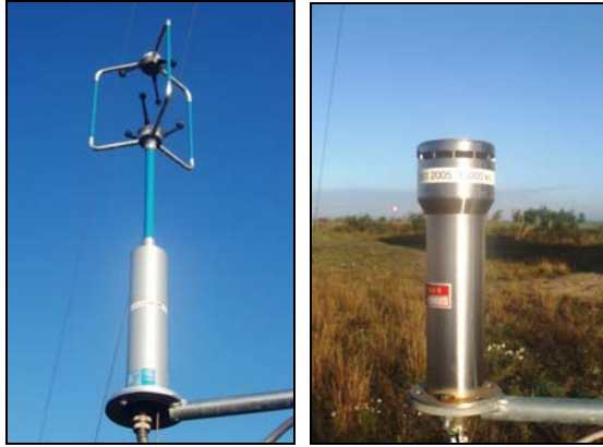
Figure 44. The 3D (left) and 2D(right) ultrasonic anemometer.
