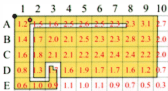
Figure 12a. The absorption and mismatch losses at 900 MHz as a function of the index finger's location on the handset's back-top region for the "firm" grip style, Antenna 1 (PIFA).
