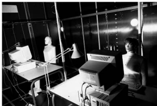
Figure 4 - Furnishings and heat load in the full-scale room. The heat load consists of two PCs, two desk lamps and two manikins producing a total heat load of 480 W.
