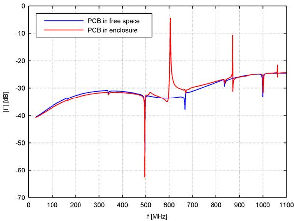
Fig. 3. Resonances of the PCB in free space (blue) and in the enclosure (red).
