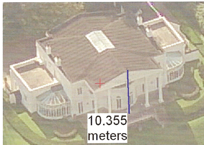
Fig. 7: Height measurement of a house.
