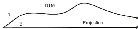
Fig. 6: Distance tool of the “EFS” software – Option 1: “Walk the earth distance”, option 2: “Flat distance” (PICTOMETRY INTERNATIONAL CORP. 2002).
