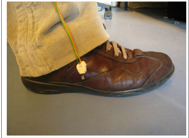
Figure 1: The contact microphone attached to the shoe.
