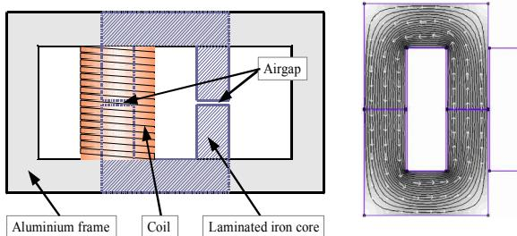
Fig. 2 On the left is shown two u-cores with an 0.8 mm air gap, and a coil to excite this core with 80 turns and 3 mH inductance. The core has a cross sectional area of 6 cm<sup>2</sup>. The acceleration sensor is placed on the aluminum frame. The right side is a result from a FEM simulation of the magnetic circuit.
