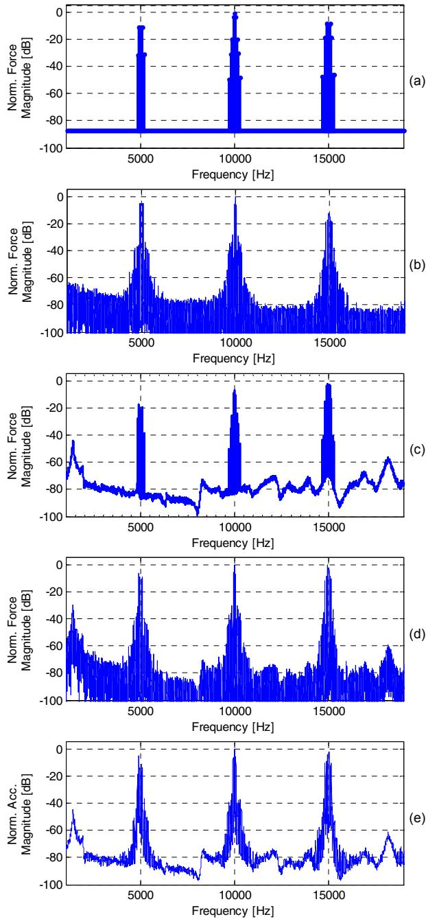
Fig. 5 The normalized vibration spectra on the frame of the coil: (a) analytically calculated spectra, (b) spectra derived using the current to force look-up table, (c) analytical calculated spectra adjusted with the transfer function of the mechanical structure, (d) Simulation using force look-up table adjusted with the transfer function of the mechanical structure (e) measured spectra
