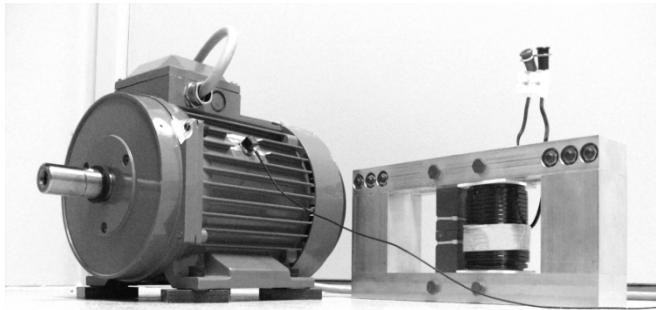
Fig. 1 The motor and coil used for measurements
