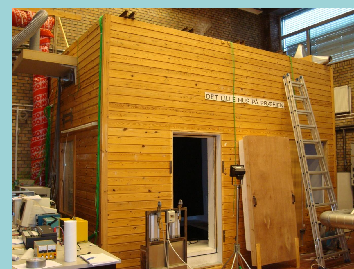
Full-scale test room 3.17 m (L) × 2.64 m (W) × 2.93 m (H)
