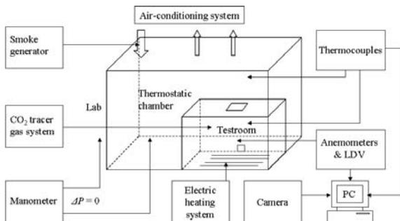
**Figure 2. Schematic representation of system and measurement equipments.**
