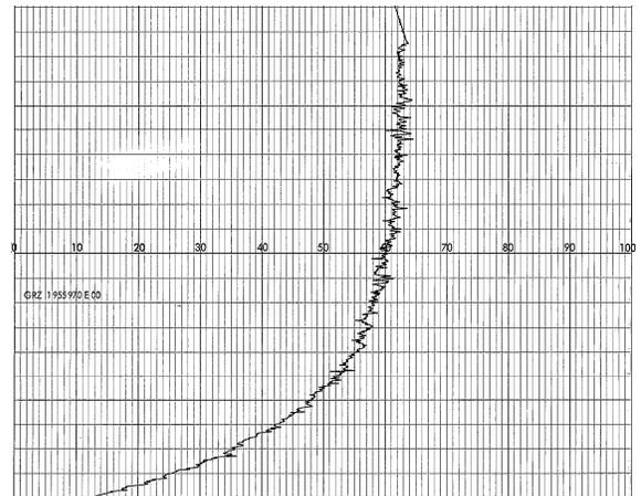
**Figure 7. The CO<sub>2</sub> concentration history at the center point of the testroom for case  $S = 0.8$ m,  $L/D = 0.147$ , and  $\Delta T = 18.7$  °C.**
