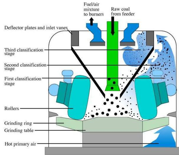
Fig. 1. Sketch of vertical spindle coal mill. The measured quantities in the mill are the inlet primary air flow  $m_{pa}$  and temperature  $T_{pa}$ , the raw coal flow from the feeder,  $m_c$  and the temperature inside the mill,  $T_m$ .
