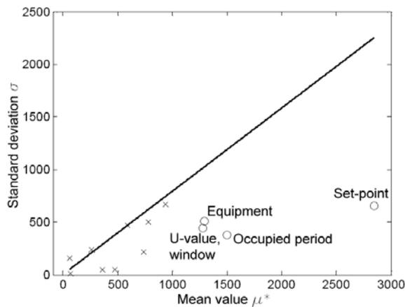
Figure 8 Screening sensitivity analysis performed using the method of elementary analysis based on 140 parameter combinations. The location of the four most important parameters are marked as circles the rest being shown as crosses, see Table 4.
