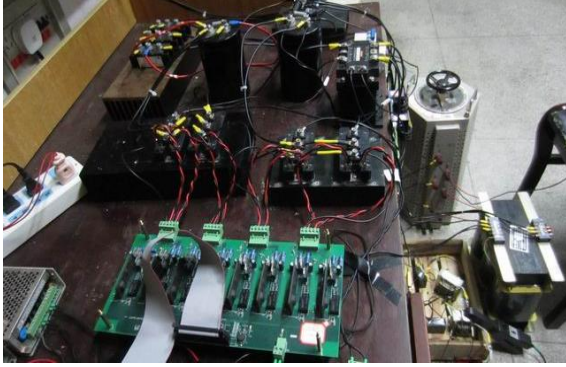
Fig.16 Prototype of parallel inverters system setup
