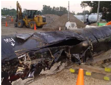
Figure 1 .Failure because of high pressure
