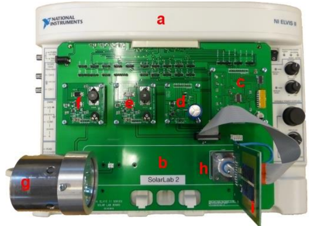
Fig. 1 Top view of the SolarLab platform: a) NI ELVIS II development board; b) custom SolarLab control and measurement board; c) stepper motor control; d) I-V characterization; e) temperature control; f) light control; g) halogen lamp; h) stepper motor; i) solar cell support including heater and sensors.
