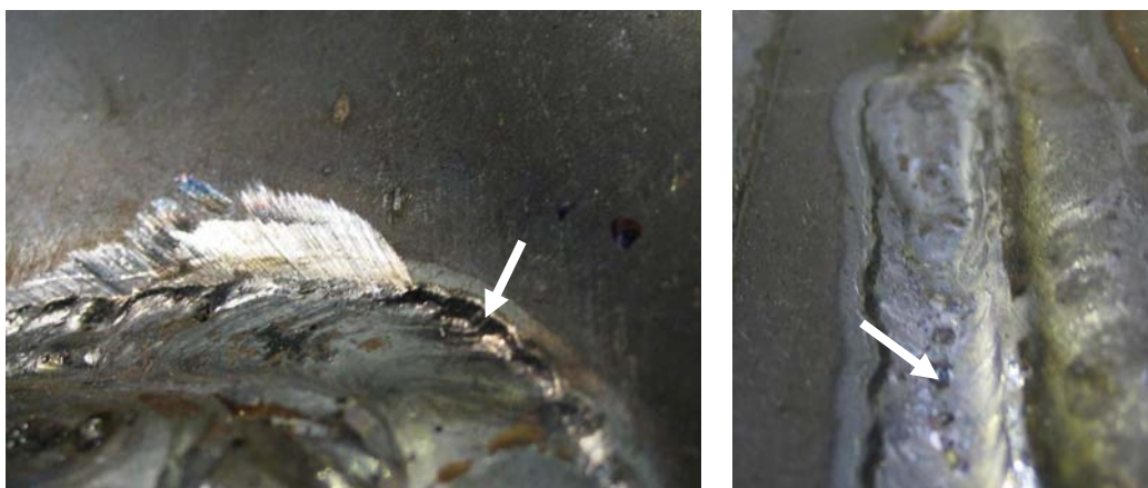
Fig. 16: Initial quality problems with TIG dressing.
