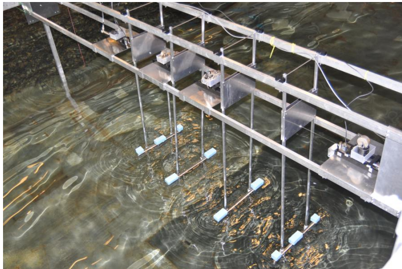
Figure 3: Picture of the WavePiston model during the tests in the lab.
