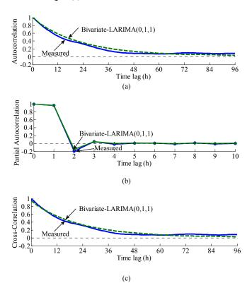
Fig. 2. Bivariate-LARIMA(0,1,1) model (dashed) versus measurements (solid): (a) Sample autocorrelation, (b) partial-autocorrelation, and (c) cross-correlation coefficients
