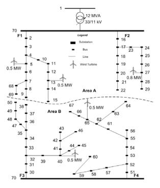
Fig. 7. The case network modified from the 69-bus distribution system [24].
