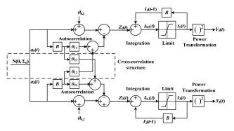
Fig. 1. Block diagram of the bivariate-LARIMA(0,1,1) model.
