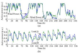
Fig. 8. Simulated time series of two weeks: (a) wind power generation, (b) load.
