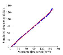
Fig. 3. Quantile-Quantile plot of the simulated time series from the bivariate-LARIMA(0,1,1) model against the measured time series (dashed), and straight line with unit slope (solid).
