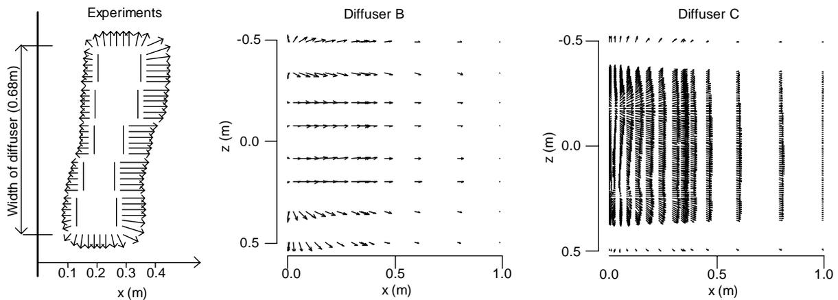
**Figure 7** Illustration of horizontal flow pattern near the diffuser from experiments and diffuser model B and C.
