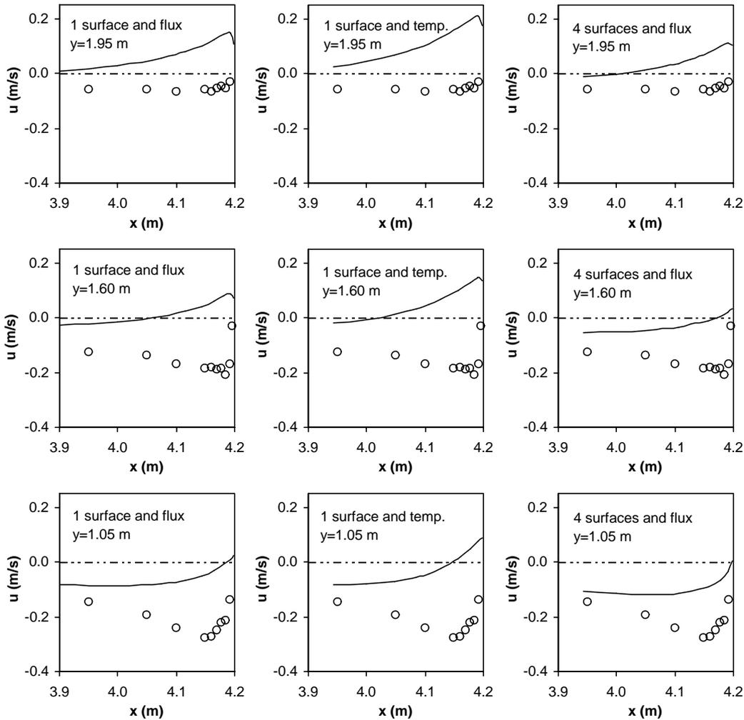
**Figure 11** Velocity profiles near the heated surface. The profiles shown are the average profiles at a given  $y$  position from experiments (O) and corresponding CFD results (line). Positive velocities indicate an upward flow.
