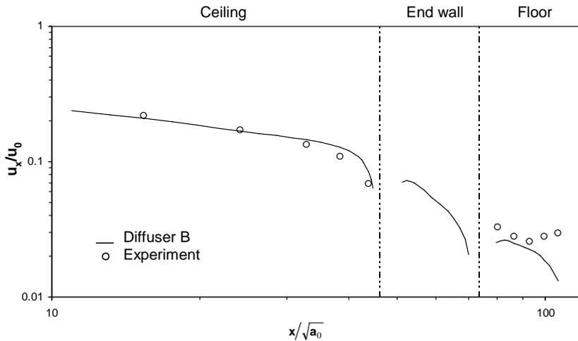
**Figure 10** Velocity decay in the recirculating flow for diffuser B (line) compared to experimental results (O).  $u_x$  is the maximum velocity at position  $x$ ,  $u_0$  is the inlet velocity,  $x$  is the position and  $a_0$  is the effective inlet area.
