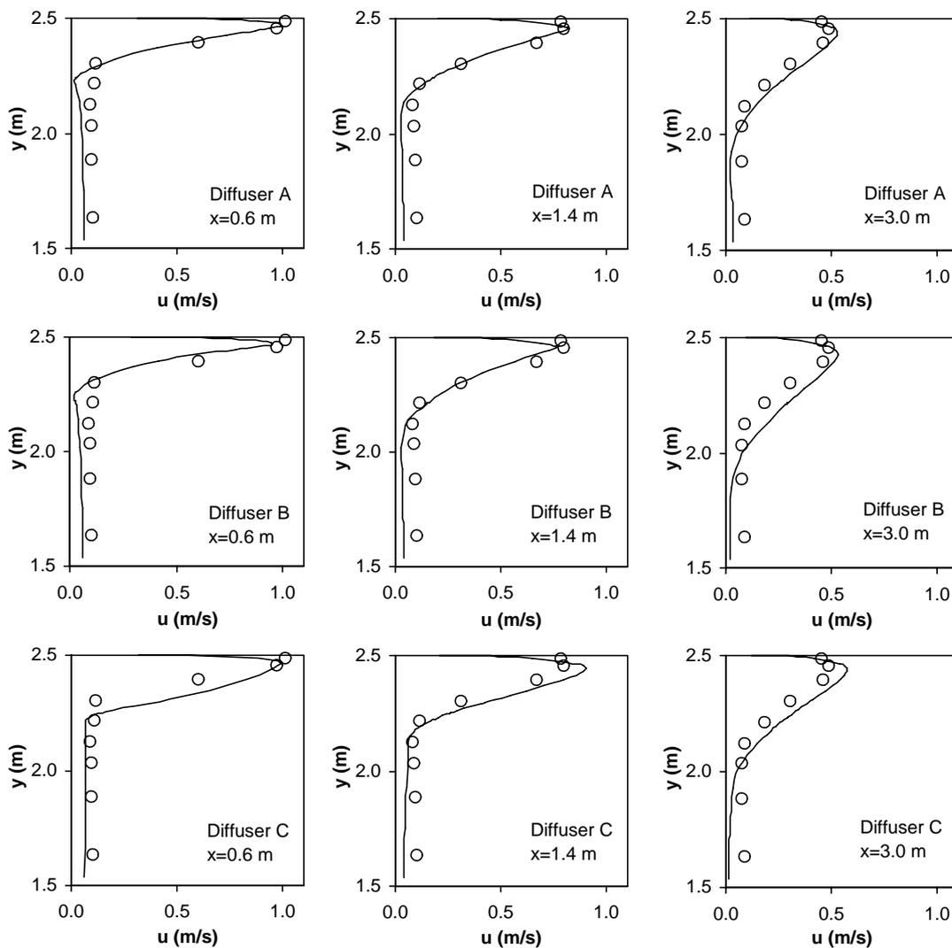
**Figure 9** Vertical velocity profiles in the jet centreline for the diffuser models (line) compared to experiments (O) at different  $x$  stations. The jet centreline for diffuser C is not identical to the room centreline due to jet asymmetry.
