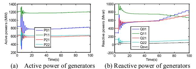
(a) Active power of generators (b) Reactive power of generators
