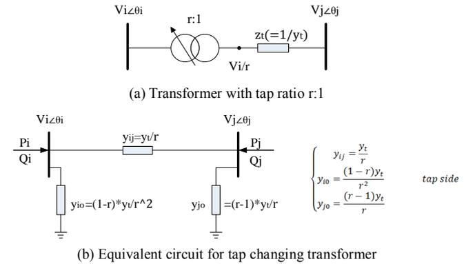
Figure 2 A transformer branch with tap changer
