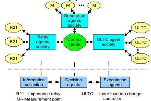
**Figure 4** The structure of MAS based control system
