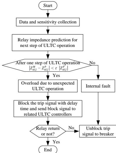
**Figure 3** Flowchart of ULTC operation induced overload identification
