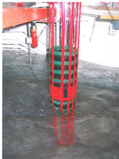
Figure 2. Picture of the mounted wave gauges.
