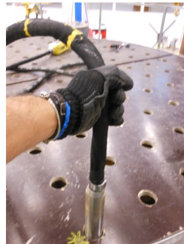
Figure 9. Vibration starts inserting the rod vibrator in the hole marked in yellow.
