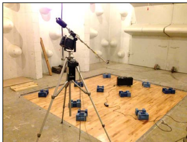
Figure 3. Test setup for laboratory measurements of impact sound improvement. The photo shows the standardized tapping machine and the floor load 25 \text{ kg/m}^2 .
