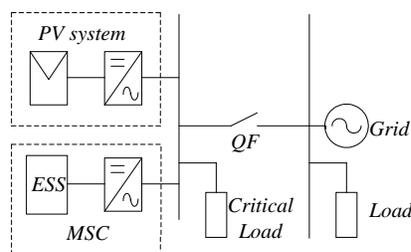
As the MSC is based on an energy storage system (ESS) and full controlled converter, it can flexibly import/export power from/to the grid. When the microgrid operates in grid-connected mode, the MSC can compensate the power variations or reduce the power fluctuations caused by the DG unit or the critical loads
