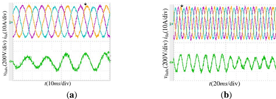
Fig.14 (a) presents the experimental results when the microgrid operates in grid-connected mode, the output power reference value of MSC is set at 2.5kW at first and then increases to 3kW. Note that its output current is increased and the output voltage is stable. During islanded mode, the MSC feed a 1.5kW load, and then another 1.5kW load is connected to the microgrid. The experimental results are given in Fig.14 (b), showing clearly that the voltage keeps stable during the whole period.
