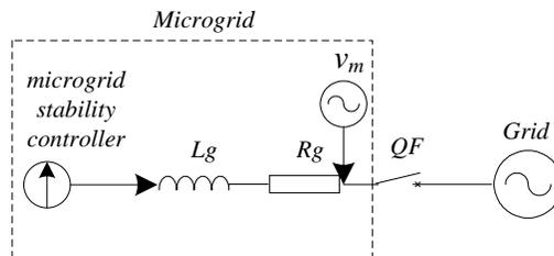
When the microgrid operates in grid-connected mode, it is connected to the utility grid at the PCC. In order to provide the desired power to the grid, we propose use the MSC to compensate power variations and
