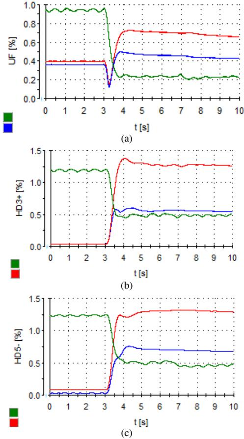
Fig. 6. Variations of voltage distortion indices: (a) unbalance factor, (b) positive sequence of 3<sup>rd</sup> harmonic, (c) negative sequence of 5<sup>th</sup> harmonic (blue: DG<sub>1</sub>, red: DG<sub>2</sub>, green: SLB).
