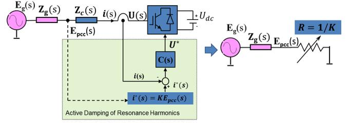
Fig. 3. Active harmonic resonance damping for STATCOM.
