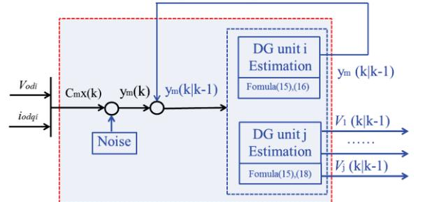
Fig.5. The proposed network voltages estimator
