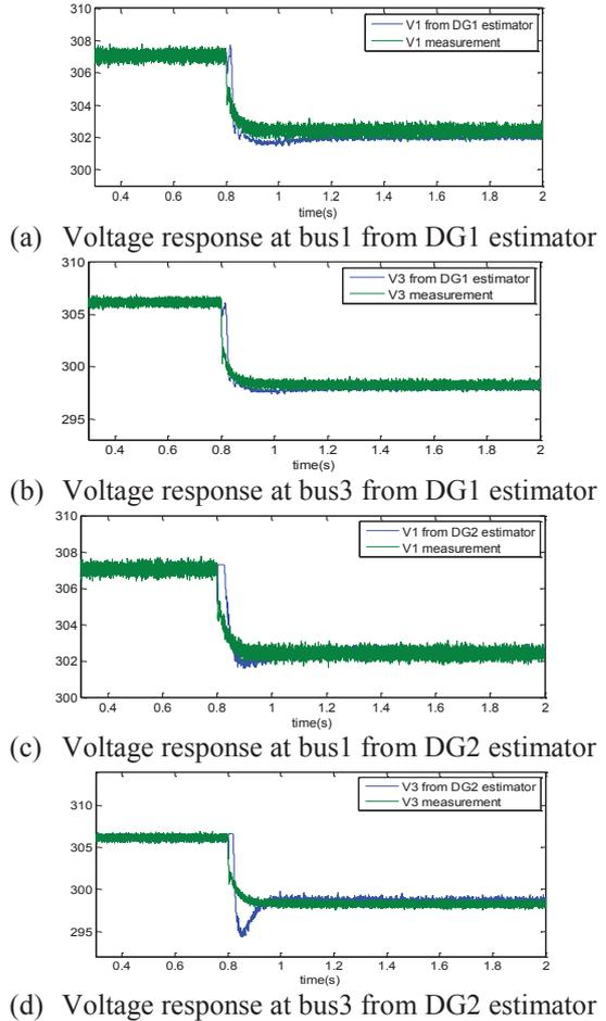
Fig.12. The simulation results for network voltage estimation.
