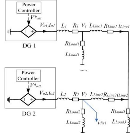
Fig.3. Small signal model of an islanded microgrid.
