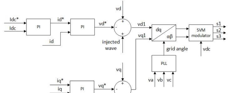
Fig. 6 - Block scheme of the boost control system
