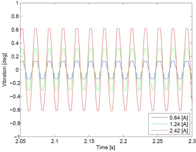
Fig. 3 - Rotor vibrations as a function of current
