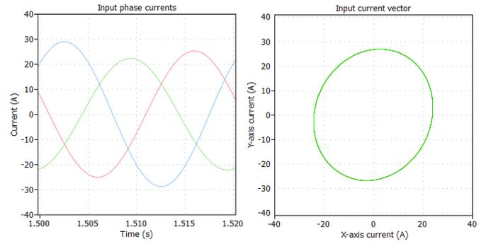
Fig. 2 - Input phase currents for the disbalanced system
