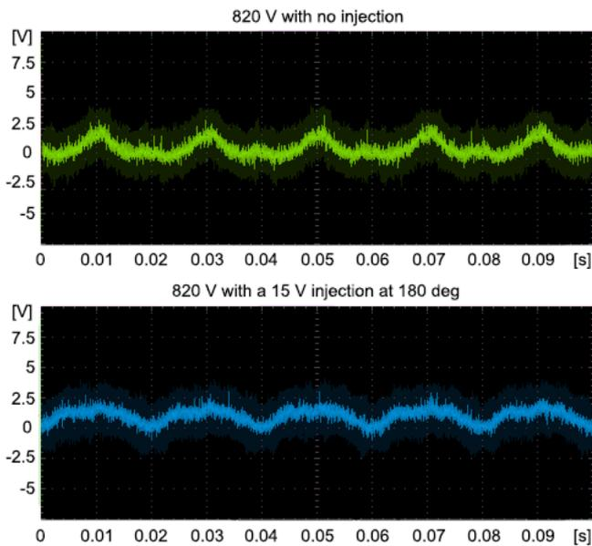
Fig. 10 - Boost mode test with the voltage DC component taken out for easier ripple visualization, upper plot shows the uncompensated response while the bottom response is compensated
