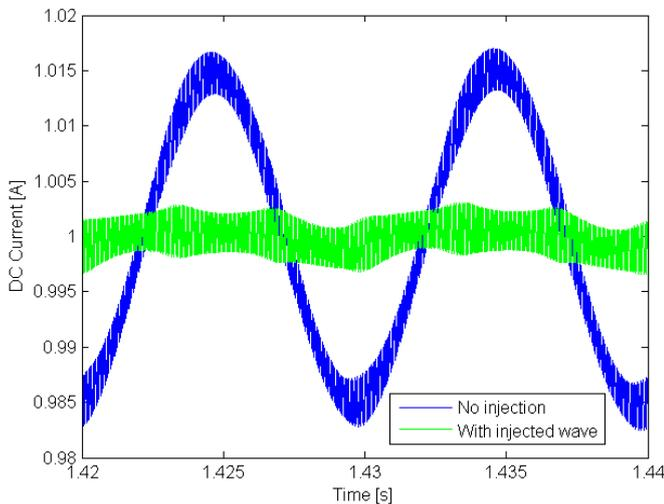
Fig. 8 - Current ripple reduction using the wave injection method
