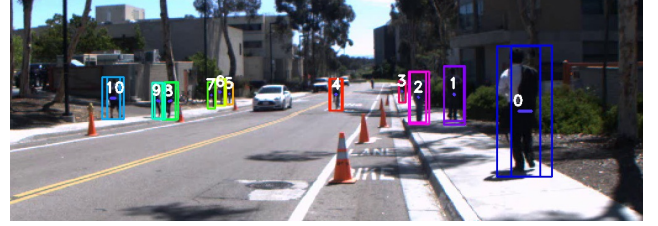
Fig. 2. Example of assignment between pedestrians. Two boxes are shown per person: the current bounding box and the previous bounding box from the pedestrian's track. Some boxes are very close to each other, and thus hard to distinguish on the picture.
