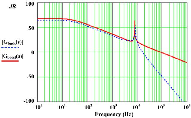
Fig. 6. Gain diagram of the control to output current transfer function.
