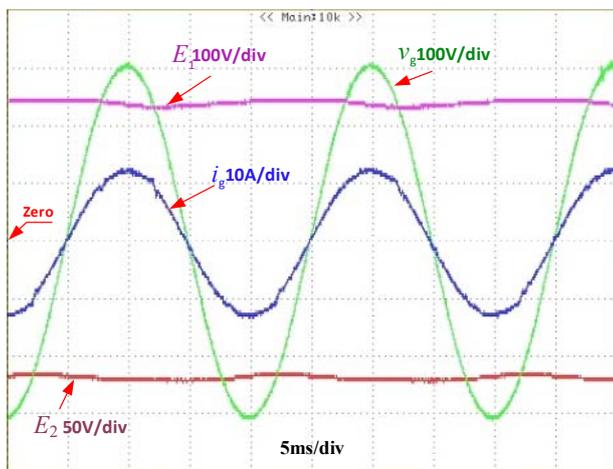
Fig. 12. Measured input DC voltages ( $E_1$ ,  $E_2$ ), grid voltage ( $V_g$ ) and grid-injected current ( $i_g$ ) in the “Buck-Boost” Mode ( $E_1 = E_2 = 240$  V).
