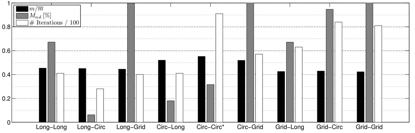
Figure 9: Graphical result overview of the original DMTO results of the 9 parameterizations with foam. The star marking at Circ-Circ\* denotes that the SLP approach has been restarted once with up-scaled  $c$  value.  $M_{nd}$  measures are truncated at 1.0%, see Table 4 for details
