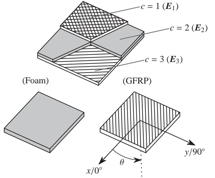
Figure 2: *Top*: Potential outcome of an example, parameterized as illustrated in Fig. 1. *Bottom*: Any unique set of material properties for the constitutive tensor  $\mathbf{E}_c$  may represent a candidate  $c$  such as for instance a foam type (left) or GFRP UD fiber mats (right), characterized by the fiber orientation  $\theta$
