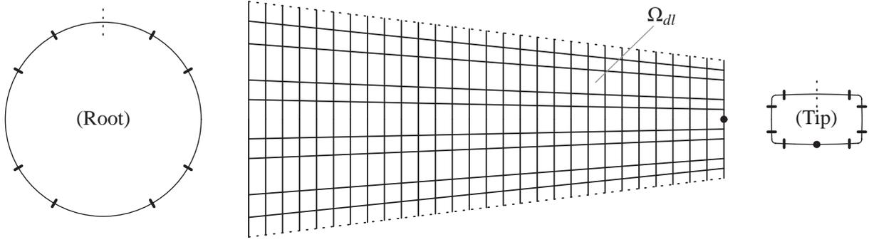
Figure 6: *Left*: Cross sectional view of the circular root section. Bold lines denote eight circumferential design domain arrangements. *Mid*: Unfolded surface view of the main spar, cut along the longitudinal direction of the upper surface. The cut is illustrated by the dotted lines. The generic main spar mesh is arranged into  $28 \times 8 = 224$  sub-domains,  $\Omega_{dl}$ . *Right*: Cross sectional view of the tip section
