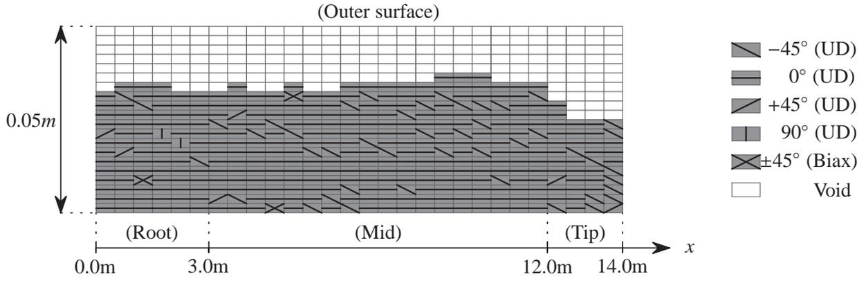
Figure 11: Rounded DMTO result of the Circ-Circ parameterization without foam. The Circ-Circ parameterization implies that the candidates are distributed in 0.5m wide circular belts, wrapped around the entire circumference of the main spar, resulting in 28 unique candidate belts throughout the length
