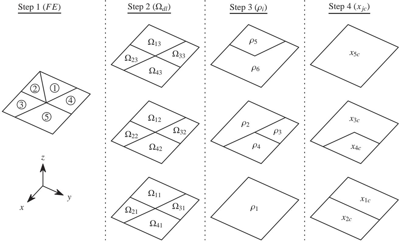
Figure 1: The design parameterization takes place in 4 steps. Step 1 concerns the finite element discretization. Step 2 concerns the arrangement into sub-domains,  $\Omega_{dl}$ . Step 3 and Step 4 concern the parameterizations into geometry domains,  $\rho_i$ , and candidate domains,  $x_{jc}$ , respectively
