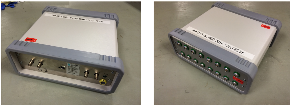
Figure 9 – Dantec 54N90 ComfortSense. Logger has 32 input channels.
