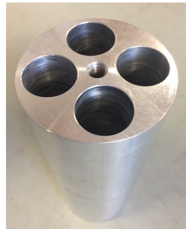
Figure 16 – Isotech Hyperion temperature bath with aluminium insert for temperature calibration of four Dantec 54R103 probes. ALS F200 Precision Thermometer is used for temperature reference.
