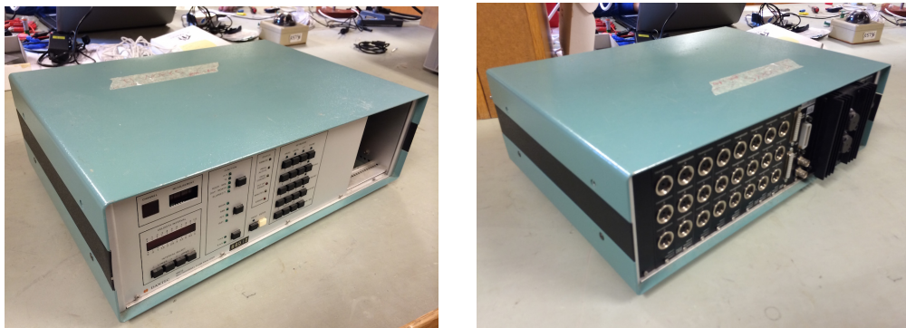
Figure 6 – Dantec 54N10 MultiChannel Flow Analyzer. Logger has 24 input channels.
