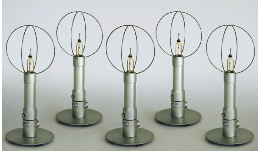
Figure 2 – Dantec Dynamics 54R10-series draught probes assembled and ready for use. Source: Dantec Dynamics A/S (2013a).
