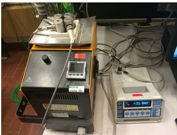
Figure 16 – Isotech Hyperion temperature bath with aluminium insert for temperature calibration of four Dantec 54R103 probes. ALS F200 Precision Thermometer is used for temperature reference.
