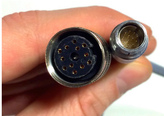
Figure 11 – Sensor cable 9054B with old plug standard in the female end (9113M0021 DIN-FATN. 12 PO) and the new standard in the male end (9113L0055 ODU Mini Snap Plug Straight).
